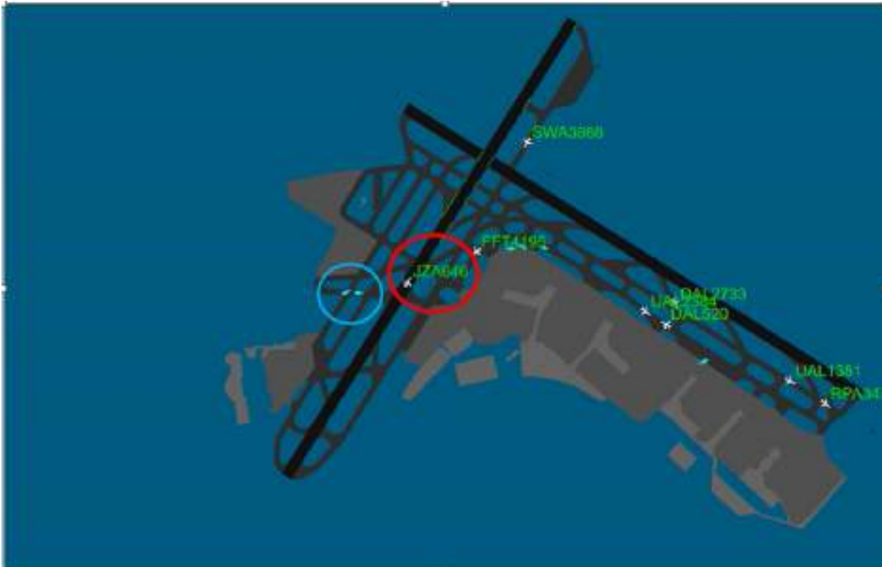
Figure 7. ADSE-X display just after the accident airplane passed taxiway D. JZA646 is the accident airplane and is shown within the red circle. The ground vehicles targets are shown in the cyan circle. (Source: FAA)
