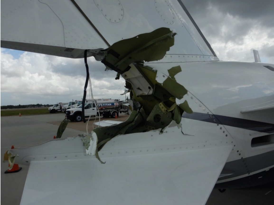
Figure 9. Right side view of N510HM's damage to its empennage.
