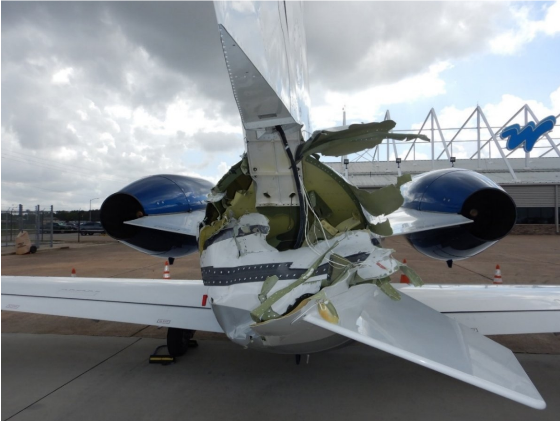
Figure 8. Aft view of N510HM's damage to its empennage.
