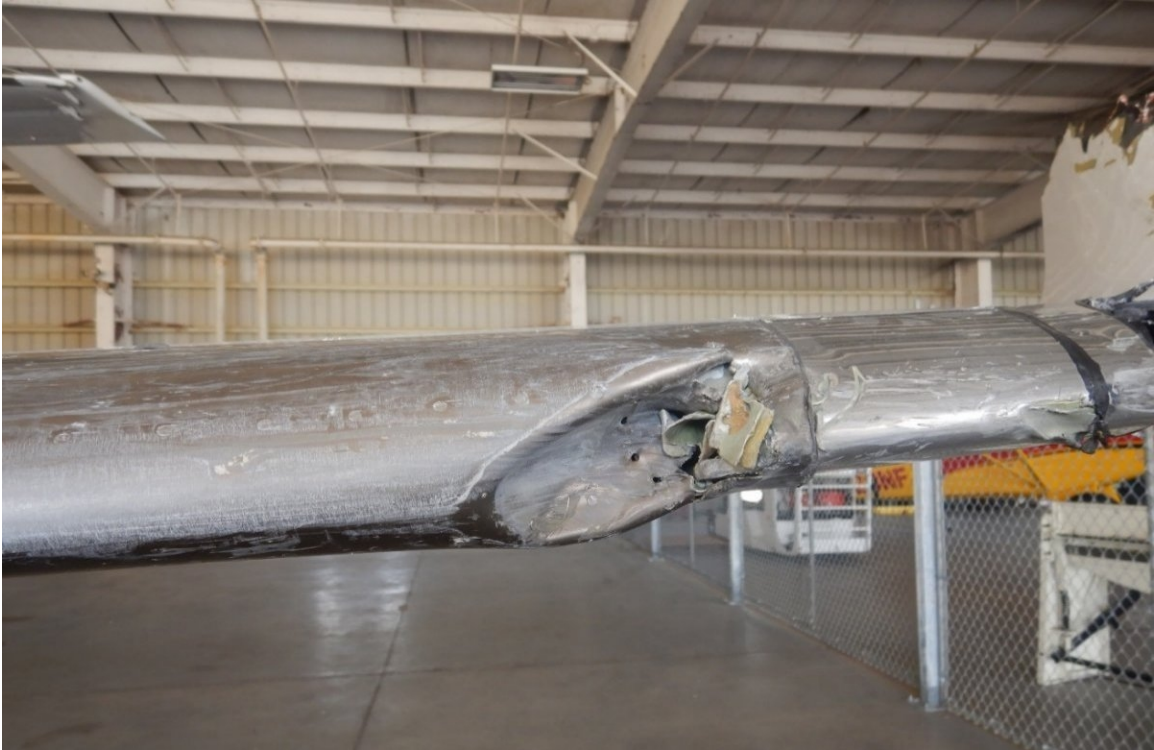
Figure 5. Close up view of N269AA's left-wing leading-edge damage.
