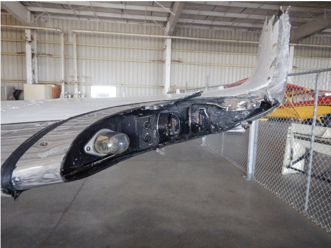
Figure 5. Close up view of N269AA's left-wing leading-edge damage.
