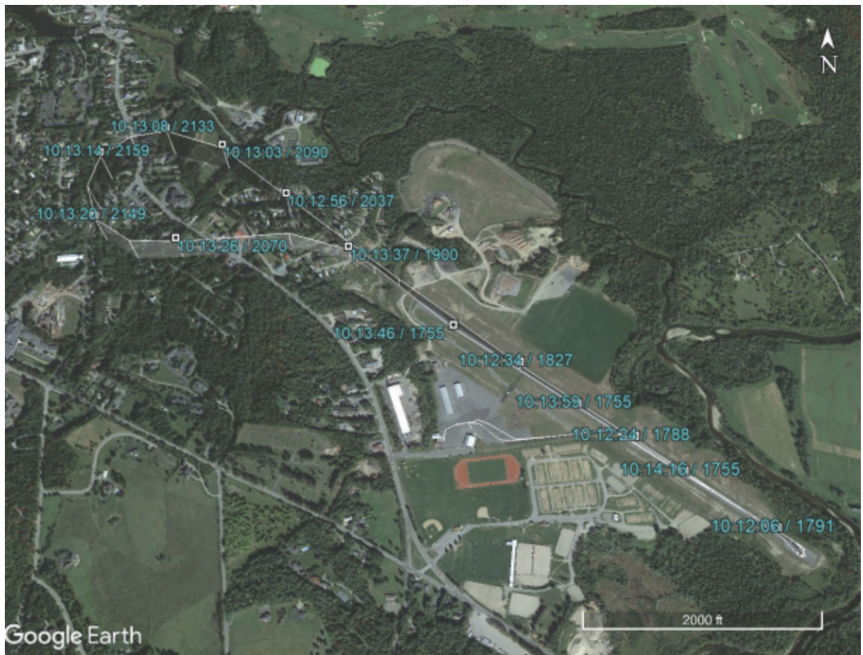
Figure 2 - Flight track for the practice flight 2 weeks before the accident flight overlaid on top of an aerial image of the airport. Annotations indicate the time (hh:mm:ss) and recorded altitude (ft msl).
