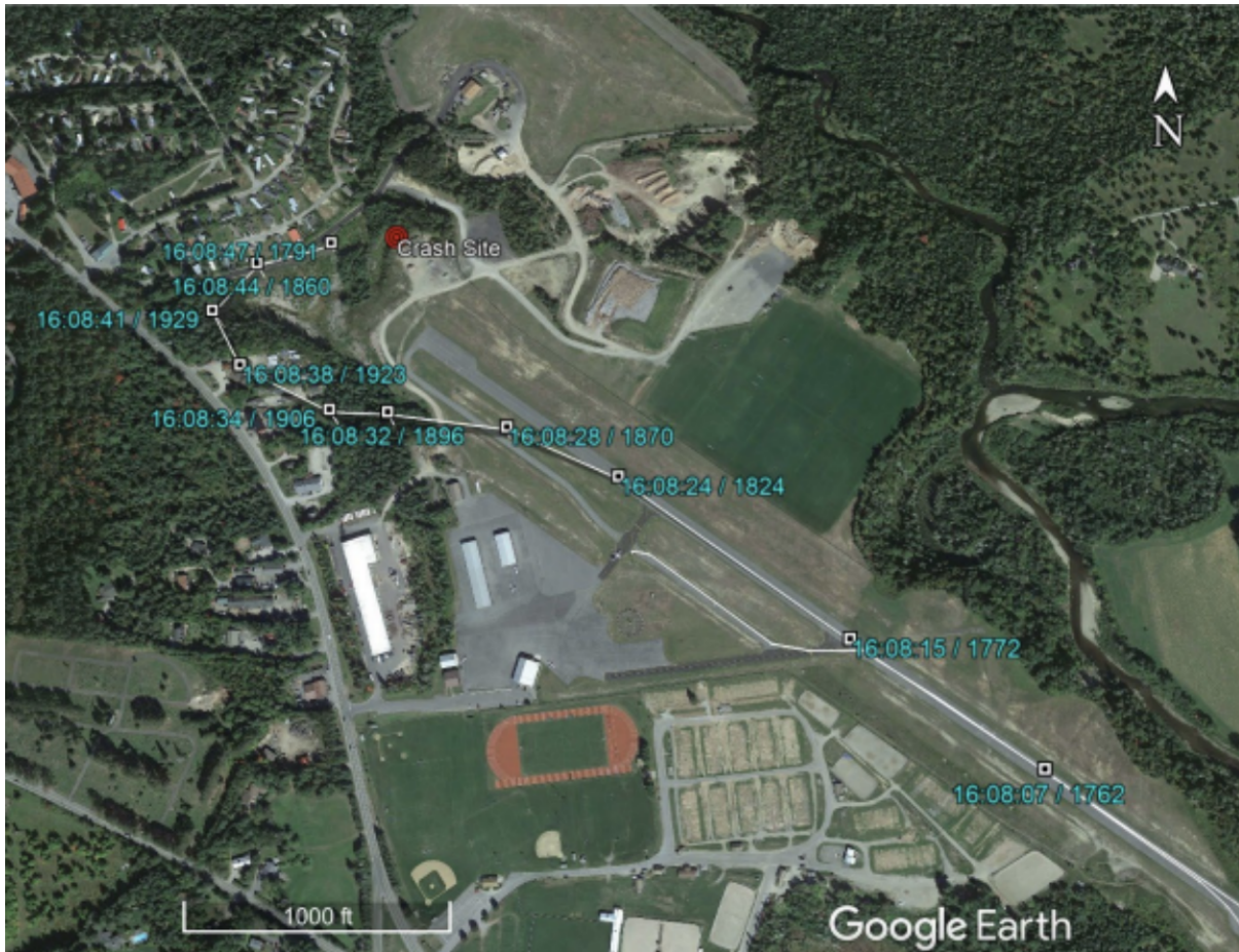
Figure 1 - Overhead view of the accident flight path overlaid on top of an aerial image of the airport. Annotations indicate the time (hh:mm:ss) and recorded altitude (ft msl). The crash site is indicated by a red circle.
