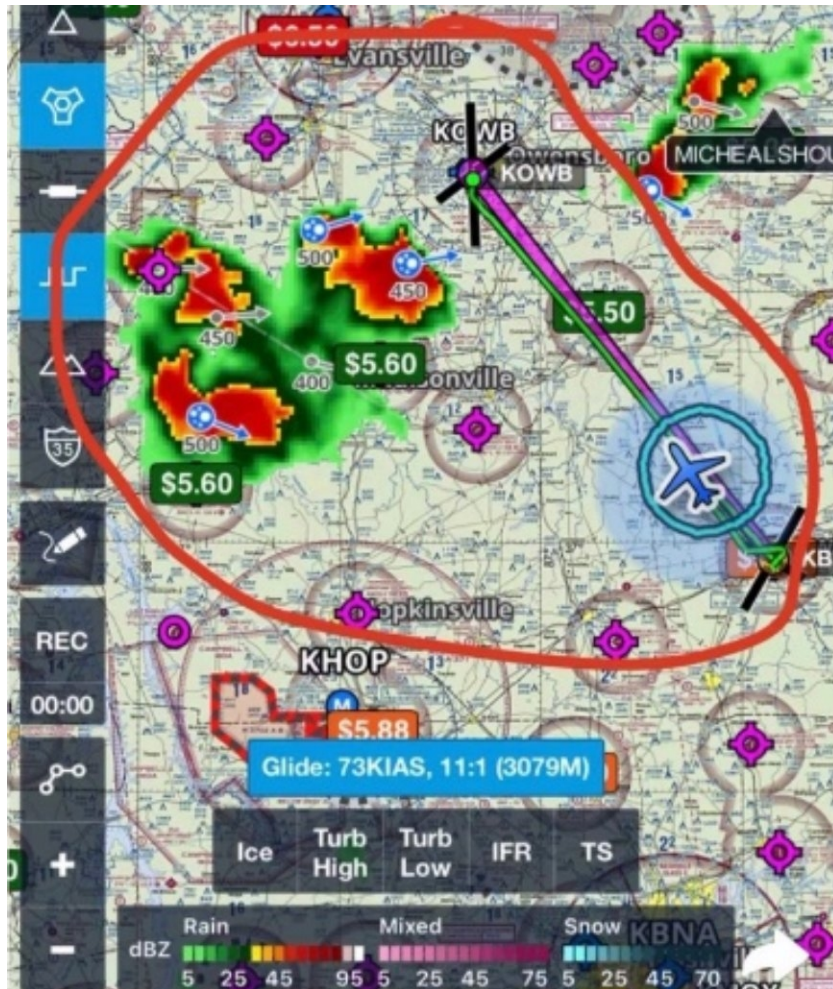
Figure 1 - Screen capture of a post to the flight instructor's social media account. Note the airplane's current position (blue airplane icon), the planned route of flight (magenta line), the depicted weather radar imagery, and entire area circled in red.
