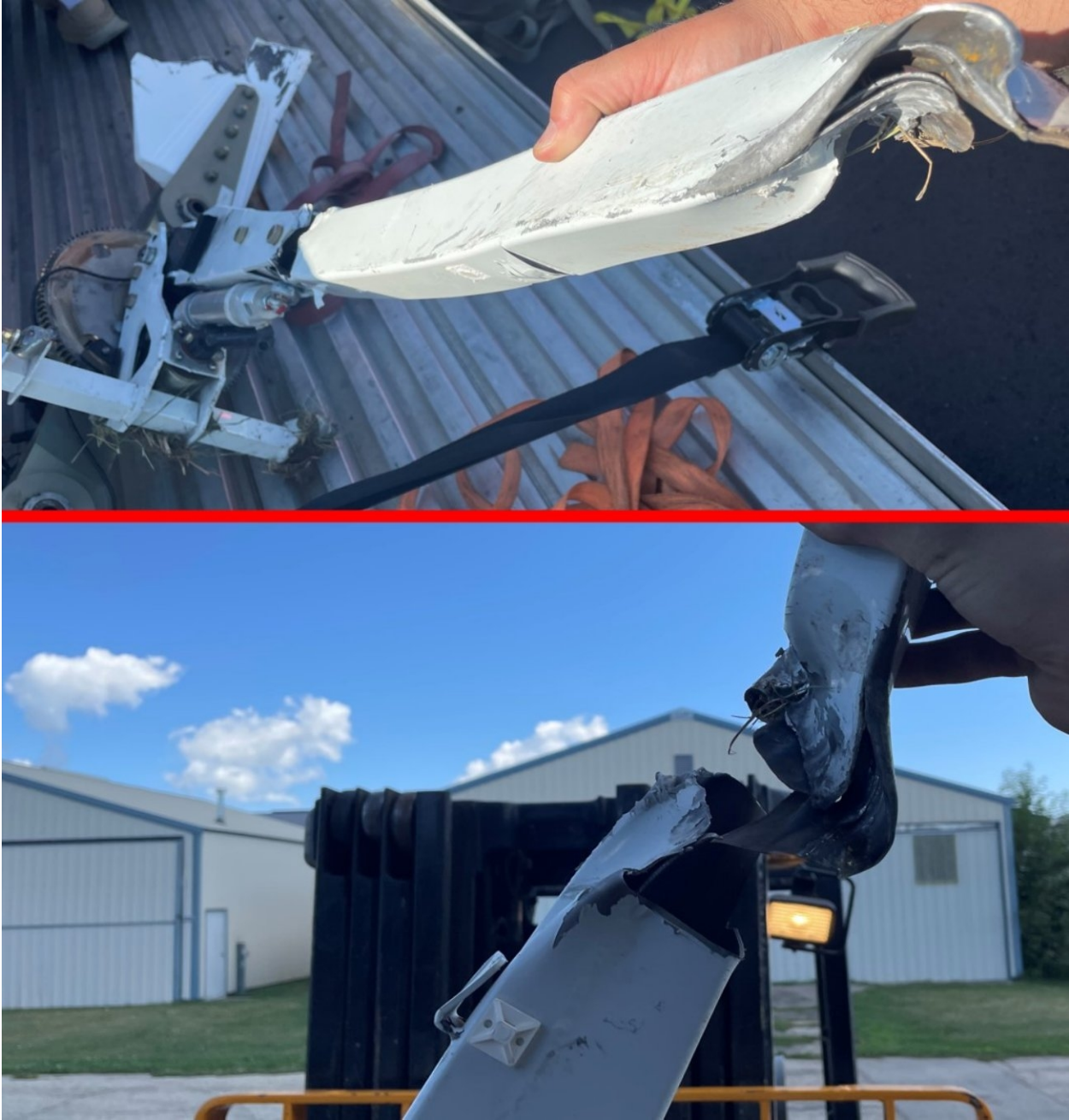
Figure 6. Gyroplane's separated rotor mast section and the helicopter's main rotor blade contact witness mark.
